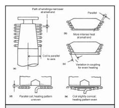
Fig. 8: Adjustment ("characterization") of induction heating patterns for several parts by varying the coupling distance or turn spacing (from F. W. Curtis, *High Frequency Induction Heating*, McGraw-Hill, New York, 1950)
