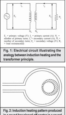
in a round bar placed off center in a round induction coil.
