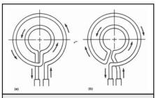
Fig. 18: Design of pancake coils to provide (a) uniform, or overall, heating or (b) peripheral heating only (from F. W. Curtis, *High Frequency Induction Heating*, McGraw-Hill, New York, 1950)
