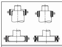
Fig. 13: Effect of coil placement on the heating pattern at the end of a workpiece (from F. W. Curtis, *High Frequency Induction Heating*, McGraw-Hill, New York, 1950)
