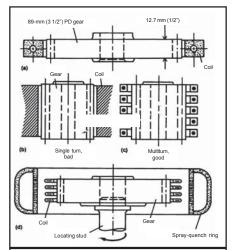
Fig. 11: Selection of single-turn vs. multiturn coils depending on the length-to-diameter ration of the workpiece (from F. W. Curtis, *High Frequency Induction Heating*, McGraw-Hill, New York, 1950)
