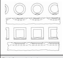
Fig. 1: Comparative heating patterns produced by using round vs. square tubing for a solenoid induction coil (from M. G. Lozinsky, *Industrial Applications of Induction Heating*, Pergamon Press, London, 1969)
