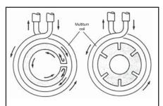
Fig. 16: Localized overheating of slots in certain parts that results from the tendency for induced currents to follow the part contour (from F. W. Curtis, *High Frequency Induction Heating*, McGraw-Hill, New York, 1950)
