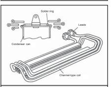
Fig. 12: Multiturn channel coil with a liner added to control the heating pattern (from F.W. Curtis, *High Frequency Induction Heating*, McGraw-Hill, New York, 1950
