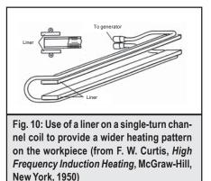
heat under the center leg as in each of the return loops. With proper balancing, the high-heat path can then be extremely narrow, while the heat produced in each of the return legs is insufficient to affect the remainder of the part.
