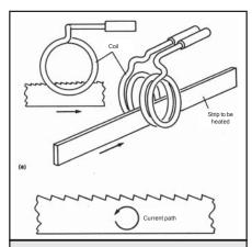
Fig. 8: Illustration (a) of one type of transverse coil for heating a thin section; sketch in (b) indicates the current path in the workpiece (from F. W. Curtis, *High Frequency Induction Heating*, McGraw-Hill, New York, 1950)
