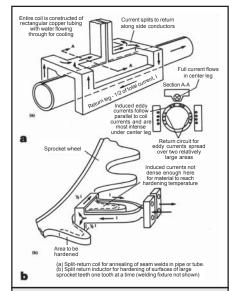
Fig. 7: Two types of split-return coils (from C. A. Tudbury, Basics of Induction Heating, Vol. 1, John F. Rider, Inc., New York, 1960)
