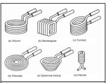
Fig. 5: Multiturn coils designed for heating parts of various shapes: (a) round; (b) rectangular; (c) formed; (d) pancake; (e) spiral-helical; (f) internal (from F. W. Curtis, *High Frequency Induction Heating*, McGraw-Hill, New York, 1950)
