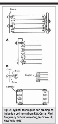
ness, and protection, it is sometimes desirable to encapsulate work coils in a plastic or refractory material. The same kind of care with respect to voltage and temperature characteristics must be taken with these materials as with insulating boards. For low-temperature induction heating applications, epoxy encapsulation of the coil is quite common. For heating of steel billets, coils are usually cast in a refractory cement to prevent scale from the part from falling between the
