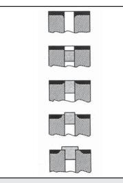
Fig. 15: Control of the heating pattern at a hole through use of copper slugs (from M. G. Lozinski, *Industrial Applications of Induction Heating*, Pergamon Press, London, 1969)
