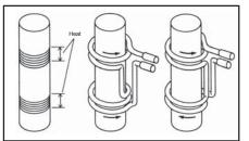
Fig. 17: Control of heating patterns in two different regions of a workpiece by winding the turns in opposite directions (from F. W. Curtis, *High Frequency Induction Heating*, McGraw-Hill, New York, 1950)
