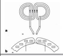
Fig. 6: Schematic illustration of a butterfly coil: (a) coil construction (arrows indicate reinforcing type of curent flow in coil); and (b) coupling between the turns of the coil and the end of a bar to produce a uniform heating pattern
