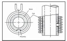
Fig. 14: Localized overheating of sharp corners, keyways, and holes most prevalent in high frequency induction heating (from F. W. Curtis, *High Frequency Induction Heating*, McGraw-Hill, New York, 1950)
